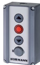
Push button DTH RM For separate control of both operational directions, with separate stop button. With miniature lock: Operator is deactivated. It is not possible to actuate the operator (2 keys included in the scope of delivery). Protection category: IP 65 Dimensions: 90 x 160 x 55 mm (W x H x D)
